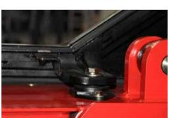
▶ There're four levels shock absorption applied to reduced the vibration from the road to the driver. The damping pad is applied reduce the vibration, Like between the steering axle and the chassis, The engine, torque convertor and the chassis, the overhead guard and the chassis. And the suspension seat is another vibration reduction.
