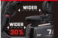
The extra foot space is provided to reduce operator fatigue significantly. The new wide-open, non-slip step makes getting in and out easy and safe.
