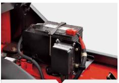
All the controllers, relays, and safety fuses are allocated in the controller box, free to water and dust. The main electronic components are waterproof, which is capable operater in severe enviroment. And the famous brand air-filter is also applied in the truck.
